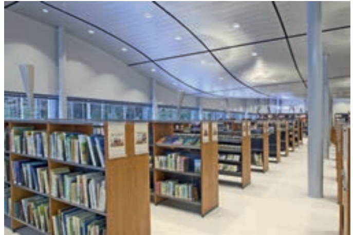
Main Library, Hollola Special curved ceiling, KSRT-300 Panel, Ral 9006.
